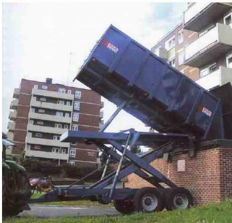
Delivering chip with a scissor lift trailer
